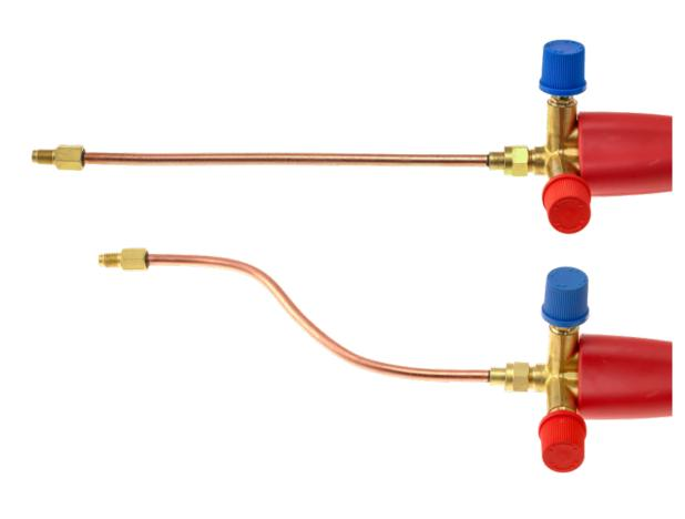
The bendable lance is an important addition to the OTS200 portable brazing kit. The lance tube is made from a special type of annealed copper that allows it to be easily and repeatedly bent into any position. This allows the operator to get the flame into areas which are difficult to reach with a normal rigid lance. This ability makes it particularly suited to plumbers and anyone doing repair work on air conditioning or refrigeration equipment.
