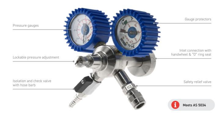
This compact regulator is specifically designed for small beer dispensing systems using  $CO_2$  and  $CO_2$  / $N_2$  mixtures. A specially designed inlet uses a hand wheel that seals easily on an 'O'-ring and a safety relief valve is fitted to the downstream low pressure side. It has high and low pressure gauges and in addition is fitted with an isolation and check valve on the outlet, which also features a multiple size hose barb.
