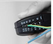
Release thumb to close stripping tool and slide to expose internal wire.
