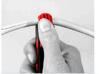
Slide stripper along cable length and peel off external sheath.
