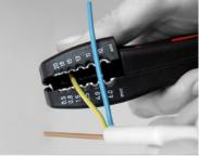
Use thumb to open spring loaded stripping tool and insert wire into appropriate stripping slot.
