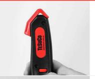
Adjust blade to external sheath depth using red finger wheel.
