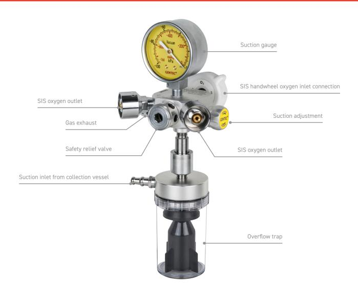
Power-Vac Series is a venturi actuated suction device which features two power take-off connectors for connecting oxygen sources. It can be used in hospital treatments, other device gas supply, life support, and any circumstances where patients require the assistant of oxygen or suction therapy. This device can be used repeatedly. The device can be connected to a central oxygen pipeline outlet or cylinder regulator with a pre-set outlet pressure.
