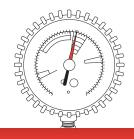
If over time the pressure gauge needle drops below the red pointer, there is a leak.
