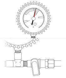
Move the red pointer so it sits above the pressure gauge needle at the pressure set.
