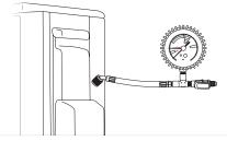
Connect the 5/16" SAE flare female nut on the test gauge to a male unit on the test piece.
