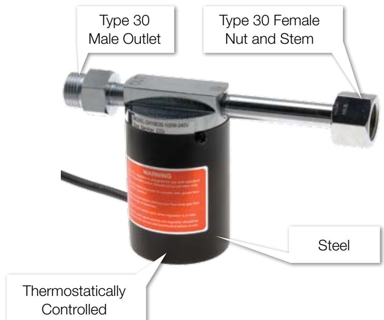
The Type 30 model gas heater is attached directly in between the cylinder and the regulator (or connection lead on manifolds) warming the gas prior to entering the regulator.
